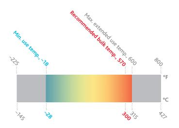
Eastman Therminol® SP heat transfer fluid is a unique, synthetic fluid designed to provide reliable, consistent heat transfer performance over a long life at recommended bulk temperatures up to 300°C (570°F).
