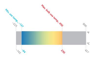
Therminol® D-12 heat transfer fluid is a liquid phase heat transfer fluid specially developed for process cooling combined with moderate heating cycles using a single fluid in place of the traditional dual steam/brine or steam/glycol systems.
